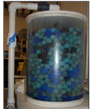
"Bio-tower" with bio-ball media; a biological filter, © S. May, NCA-PKS
