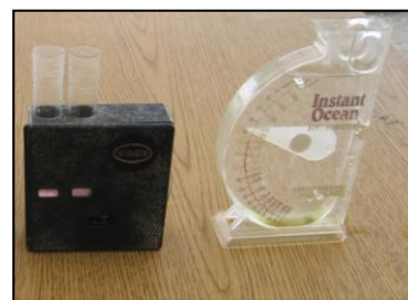
Chlorine and sat water testing equipment
