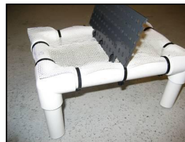
Close-up of individual float with mesh bottom and barrier
